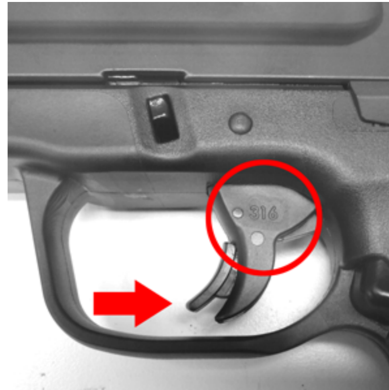
New Fast Action Trigger 316 – Safety protrudes significantly. Pistol Does Not Need Retrofit (Identified by '316' Markings)
