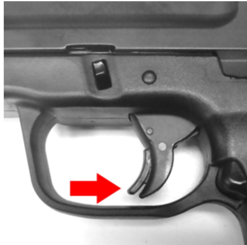
Original Fast Action Trigger – Safety protrudes slightly. Needs Retrofit!
