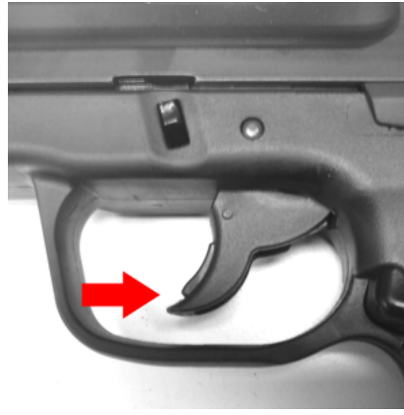
DAO Trigger can be identified by shorter trigger safety which does not break through the bottom of the trigger. DAO trigger rotates further forward. This Pistol does not need retrofit.
