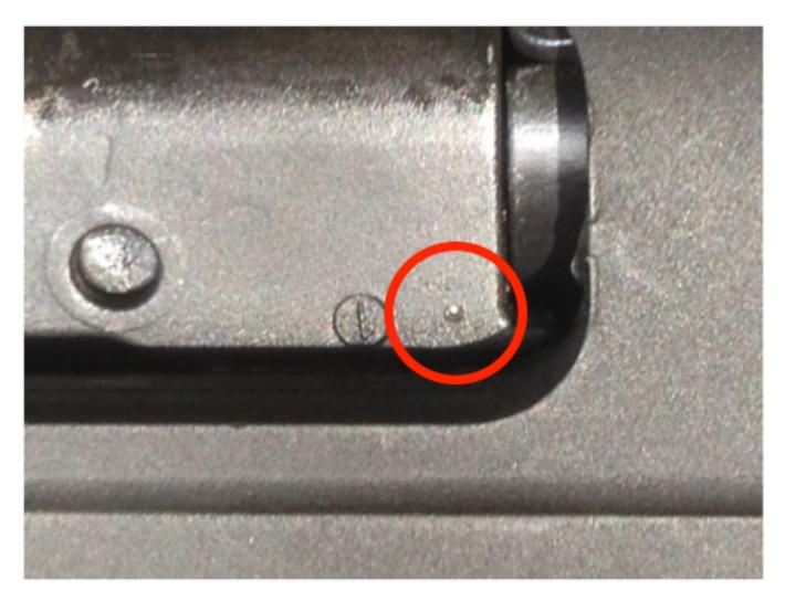
Remington has also corrected the manufacturing process to eliminate this potential firing pin problem in shotguns manufactured after November 24, 2014. Shotguns manufactured after November 24, 2014 will also have a punch mark on the bolt.
