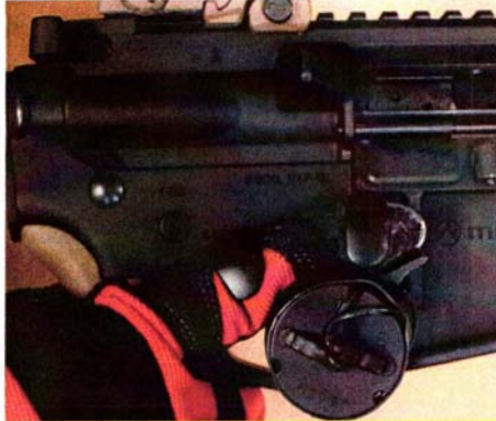
This shows the back side of the device when it is in position and ready to fire. Note that the traditional "trigger finger" is used merely to hold the device in place.
