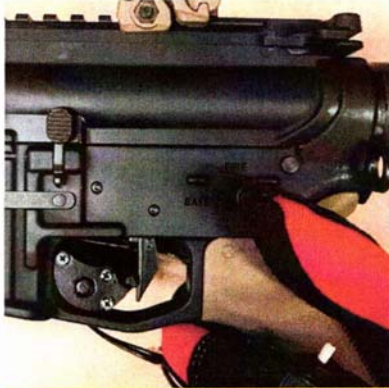
This shows the device in position and ready to fire. To fire, the shooter will move the selector to "fire," then press and hold the white activator plunger with his thumb. The firearm will fire until the thumb is released.
